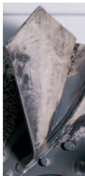
Fan wheel used in the timber industry, showing wear and tear, and with some broken off and cracked blades
