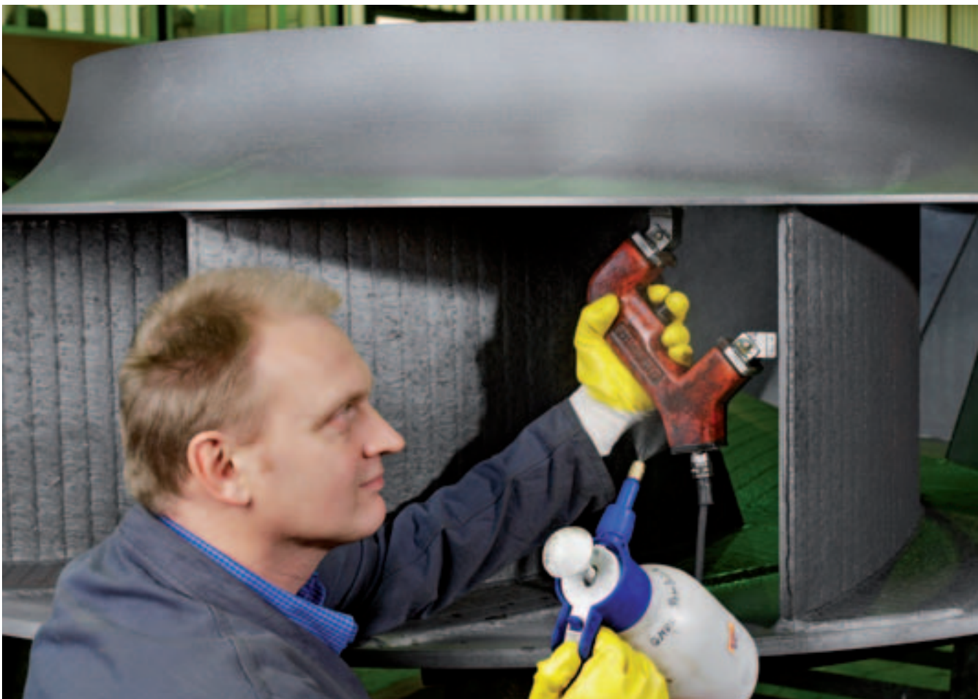
Surface crack check (MP) on the weld after the repair has been carried out
