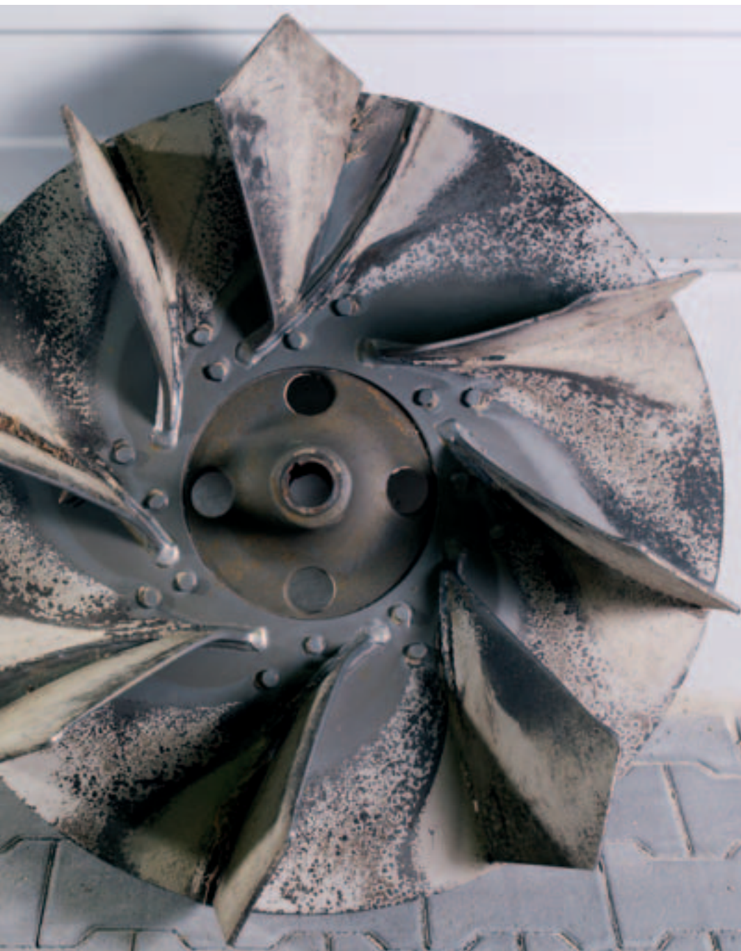
Fan wheel used in the timber industry, showing wear and tear, and with some broken off and cracked blades
