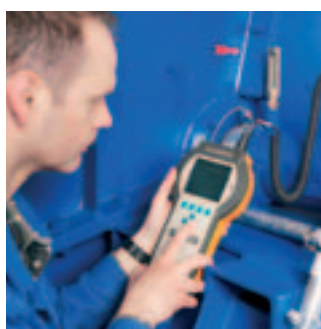
Vibration detection on a fan impeller bearing
