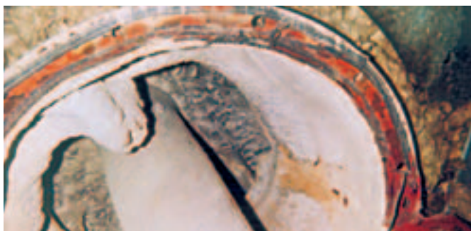
Baked-on deposits caused by the conveyance of dust-laden gases can lead to break-downs
