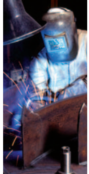
Welding work on a fan impeller under repair
