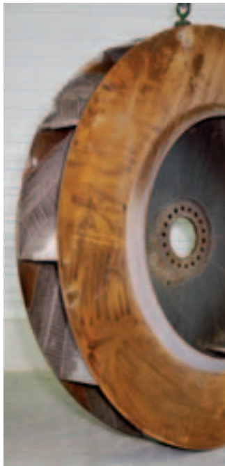
Fan impeller used in the cement industry, showing baked-on deposits and severe wear at the blade inlet edge and also on the back plate
