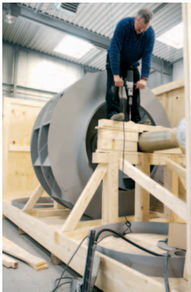
Packing a repaired double-inlet rotor in a wooden transportation frame for safe shipment
