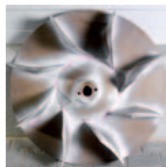
Damage analysis/ crack inspection via dye penetrant testing in the area of the stiffening cone's join with the back plate
