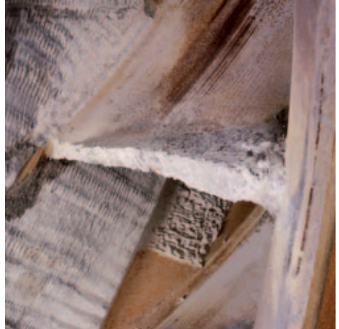
Fan impeller used in the cement industry, showing baked-on deposits and severe wear at the blade inlet edge and also on the back plate
