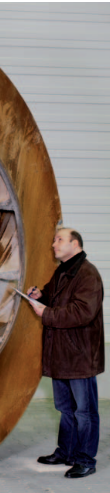
Visual check of a fan impeller in need of repair to assess the damage and prepare a cost estimate
