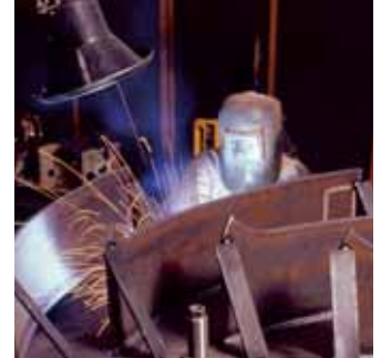
Construction of a welded impeller
