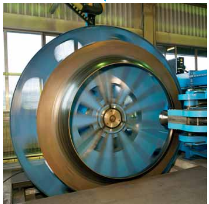
Manufacture of an impeller shroud up to 4.50 m by our stretch-forming machine
