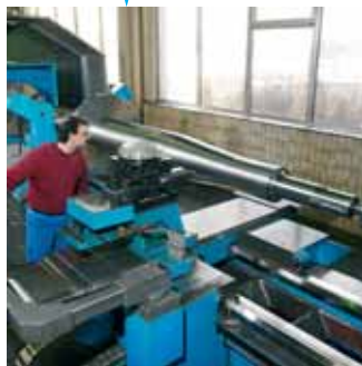
Final machining of a forged flanged shaft and a finished welded impeller
