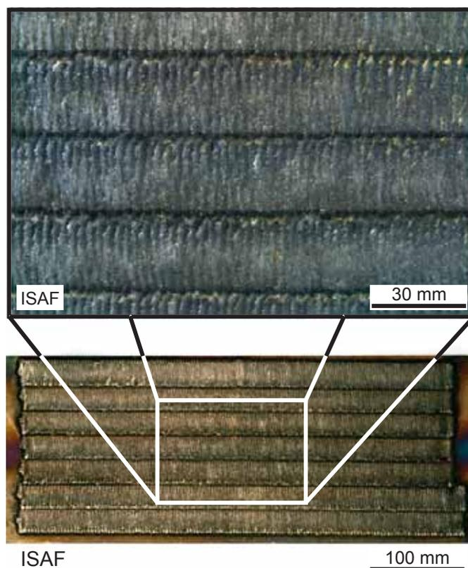
Fig. 4 Structural component coating Fe-base + Cr-Boride + VC applied by controlled dip transfer (short arc) welding process
