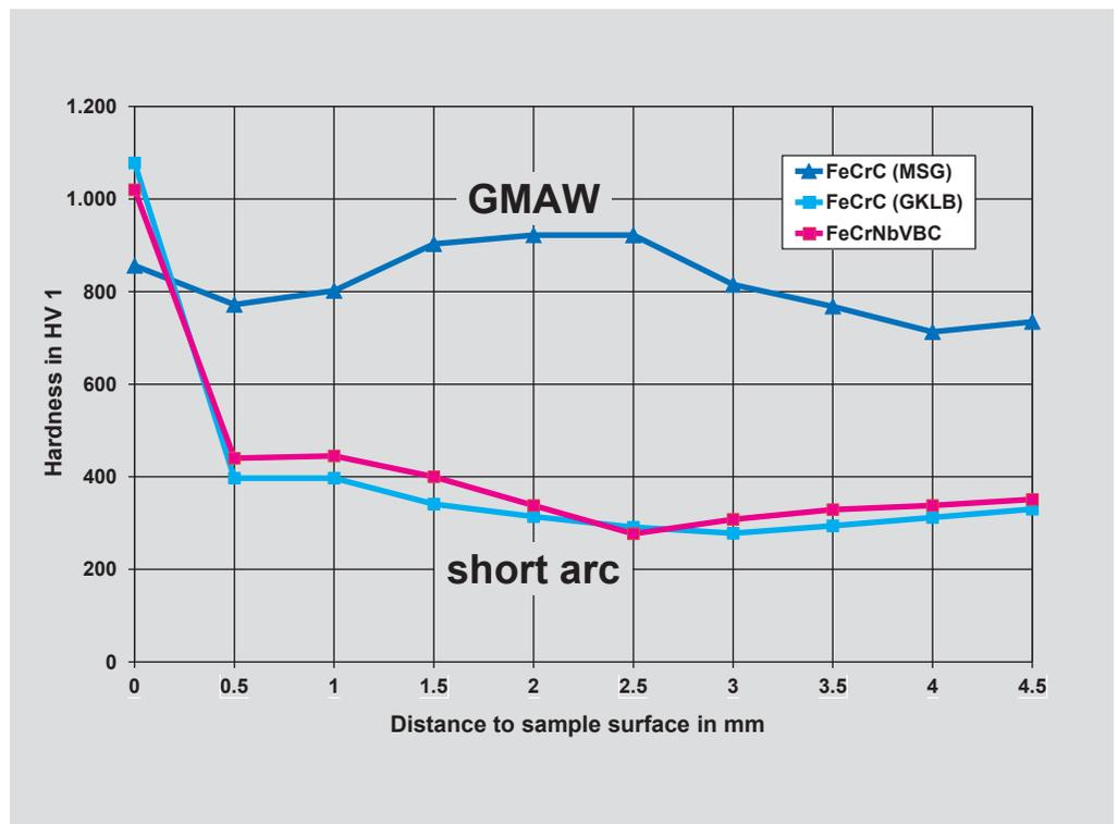
Fig. 9 Heat-affected zone hardness comparison GMAW v Controlled dip transfer (short arc) welding
