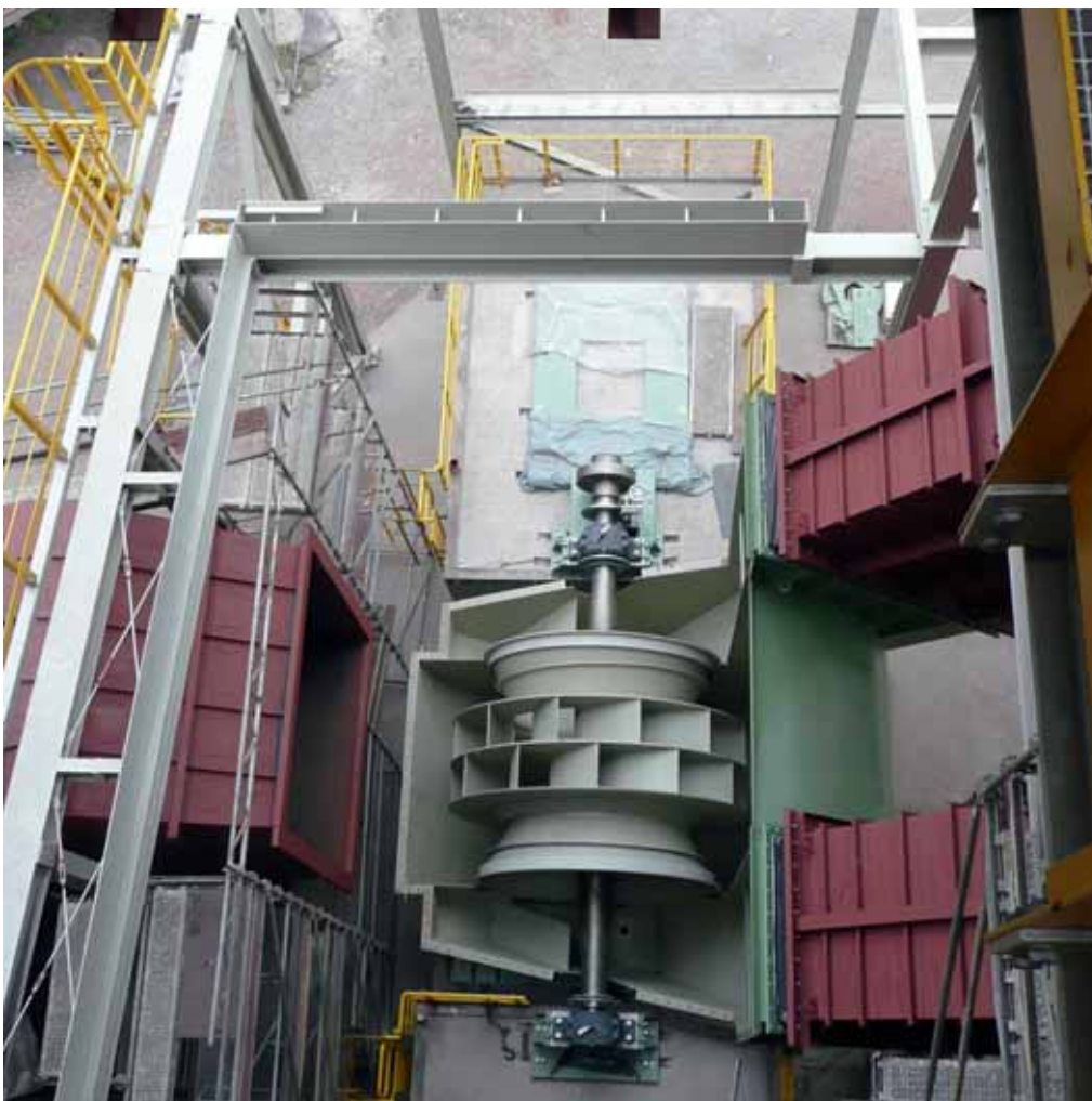
Baked-on deposits of sticky dust on the fans, caused for instance by conveying CO gas, can be kept to a minimum by targeted water injection.
